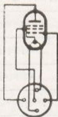
Patice O pro lampy: B 443, B 443 S, C 443, C 243N, C 443N, E 443H E 443N, F 443N
