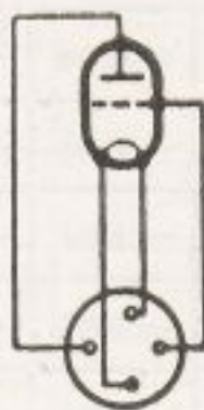
Patice A pro lampy: A 409, A 415, B 217 B 228, B 406, B 409 B 424, B 438, E 406 N E 408 N, F 410
